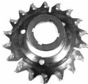
Fig.2. Sample saw destroyed due to distortion higher then ultimate
