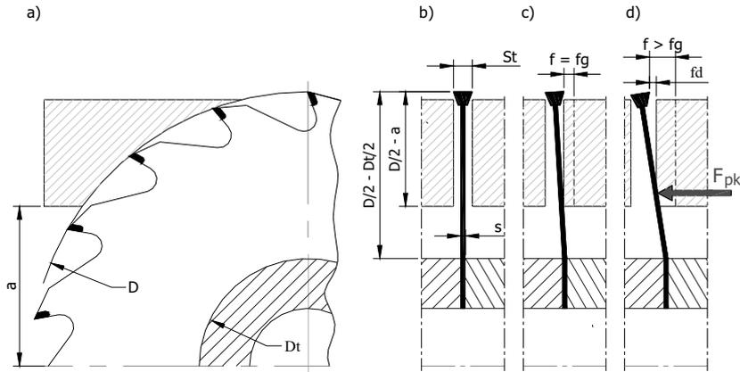
Fig.1. Distortion of the saw during cutting process, where : a) cutting scheme, b) no distortion, c) ultimate distortion, d) destructive distortion
