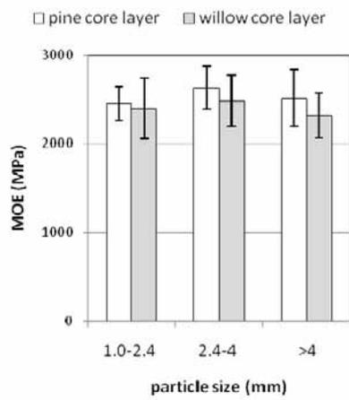
Fig. 1. Modulus of elasticity of particleboards with the core layer made from particles of different sizes
