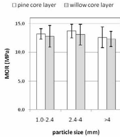
Fig. 2. Modulus of rupture of particleboards with the core layer made from particles of different sizes
