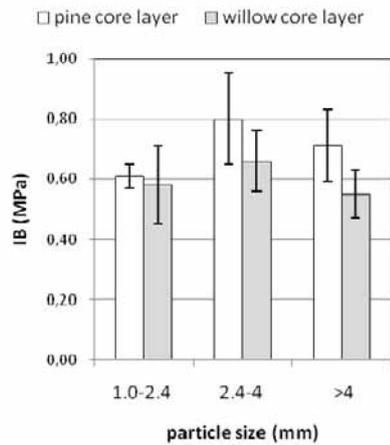
Fig. 3. Internal bond of particleboards with the core layer made from particles of different sizes
