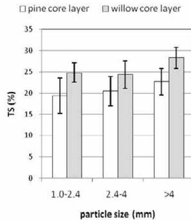
Fig.4. Thickness swelling after 24 h of particleboards with the core layer made from particles of different sizes
