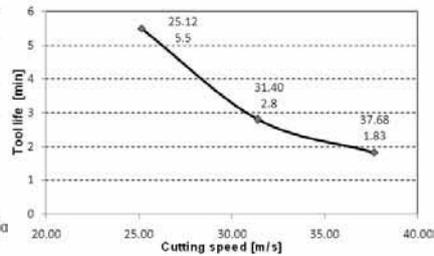
Fig. 5 Influence of the speed machining to the tool life
