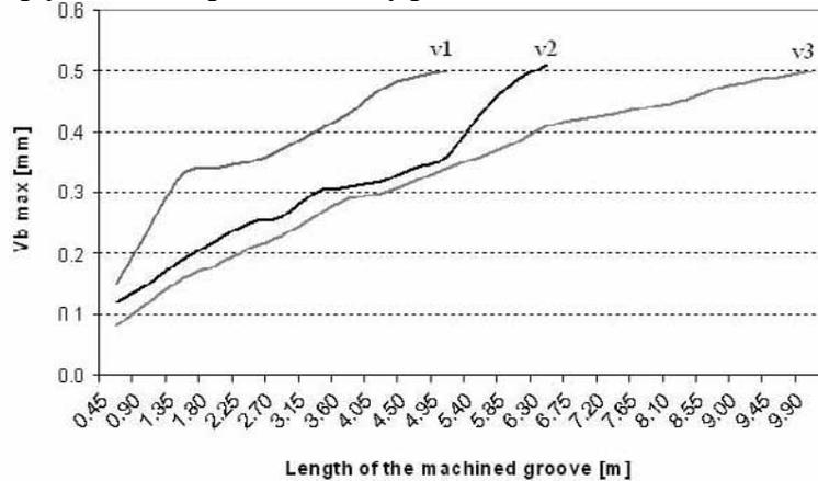
Fig.3 Course of wearing tools out in the function the way for different speeds of machining.
