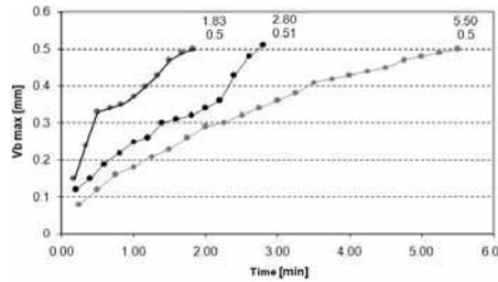
Fig. 4 Course of wearing tools out in the function of the time for of different speeds of machining
