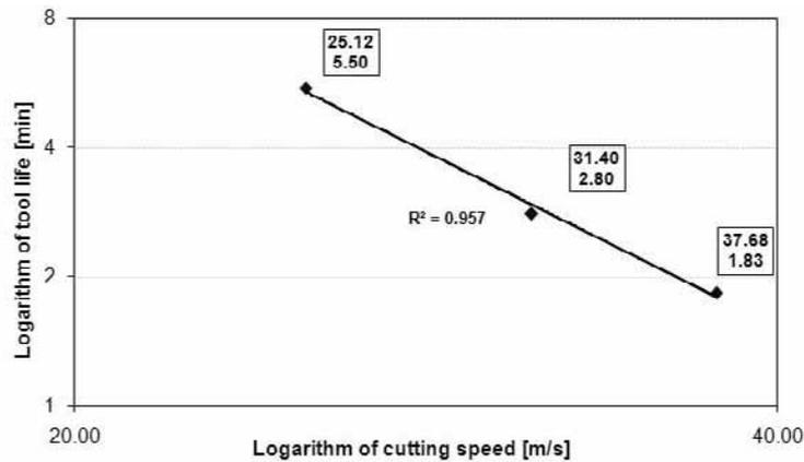
Fig. 6 Dependence of the tool life to the cutting speed.
