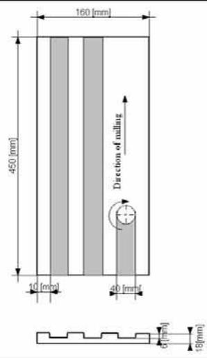
Fig. 2 Schema of the milling process
