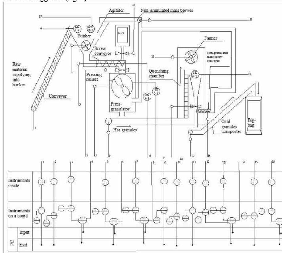
Fig.1. Scheme of automation of technological process of granulation of reduced wood raw material.
