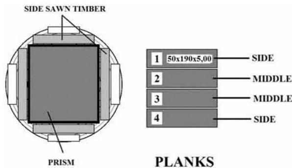
Fig.1 Transverse section across log – parts of cutting (prism, side sawn timber) and marking of planks in prism.
