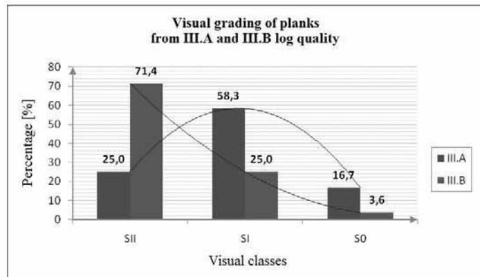
Figure 2 Visual grading of logs (III.A and III.B) and planks SII, SI and S0
