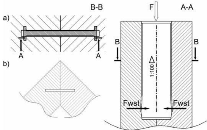
**Figure 2.** Mechanism of the development of the initial tightening: a) joint nail hammered into elements, b) kerf made in elements prior to assembly;  $F$  – hammering force of the joint nail,  $F_{wst}$  – force of the initial tightening [2]
