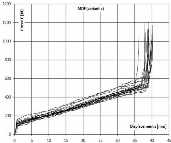
Figure 5. Results of examination of the insertion force of double-tee fasteners into MDF board without cutting (variant a)
