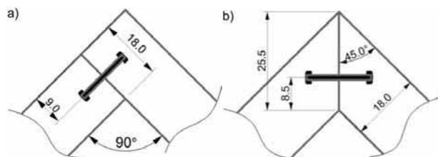
Figure 4. Variants of the experimental joints: (a) straight boards (b) skew boards.
