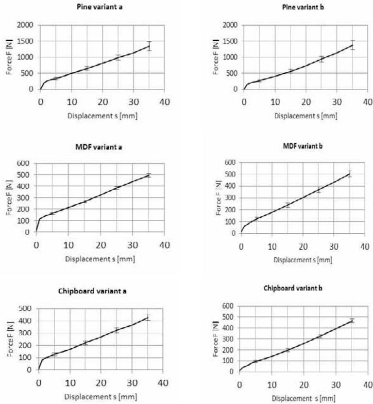
Figure 6. Results of investigations of the insertion force of joint nail type fasteners (with confidence intervals 95%) in oak, pine, chipboard and MDF of boards for straight and skew connections.
