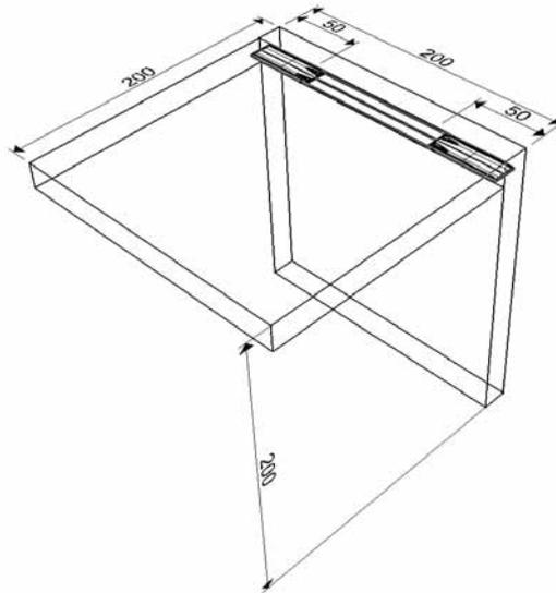
Figure 3. Spatial model of the sample used in experiments.
