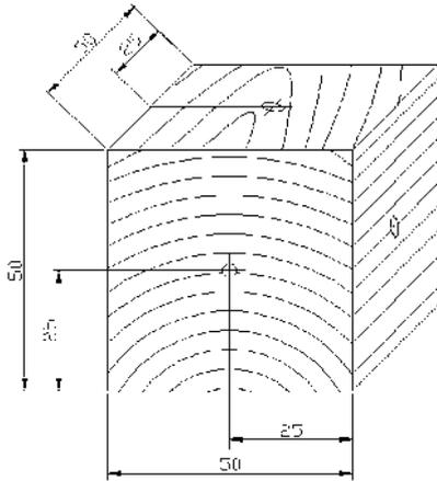
Fig. 1. Sample shape and dimensions.
