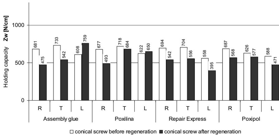
Fig. 4. Holding capacity for the conical screws set in pinewood.
