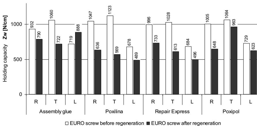
Fig. 3. Holding capacity for the EURO type screws set in pinewood.
