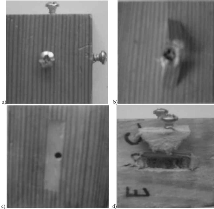
Fig. 2. Example phases of the course of the experiment: a) mounting of connectors in the sample; b) view of damaged sample; c) treatment of the damage; d) tearing out of the connector from regenerated sample.
