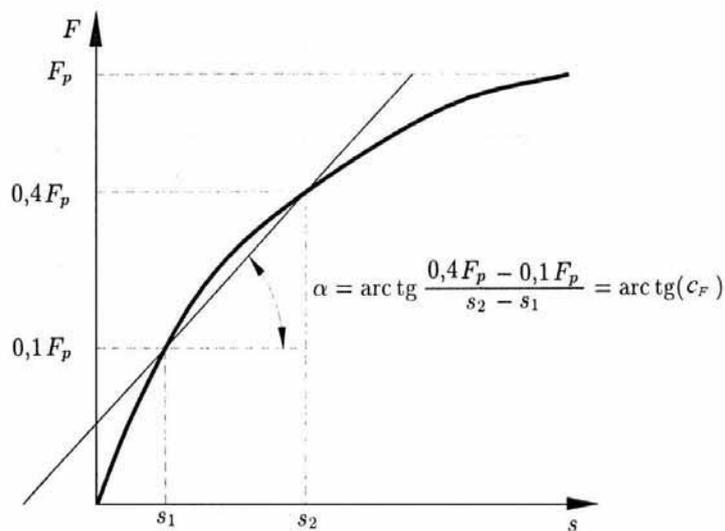
Fig. 1. Characteristics of a semirigid joint and method of determination of its rigidity (Modelowanie... 2004).
