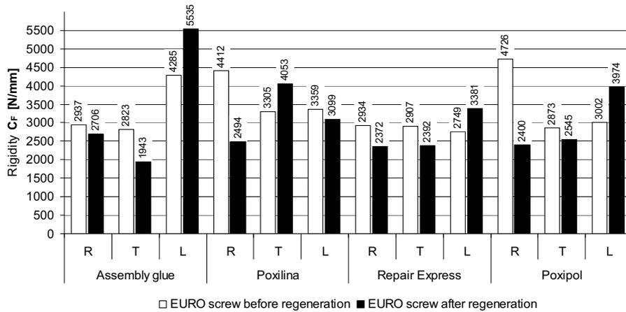
Fig. 3. Values of rigidity of the EURO screw-pinewood connection before and after regeneration using different preparations in three anatomical planes.
