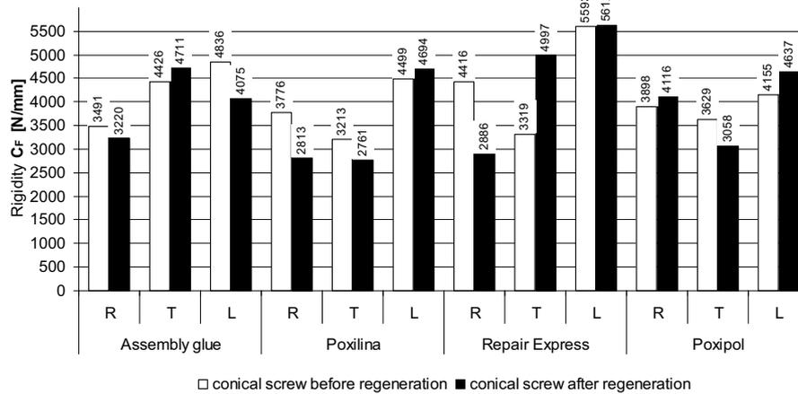
Fig. 4. Values of rigidity of the conical screw-pinewood connection before and after regeneration using different preparations in three anatomical planes.
