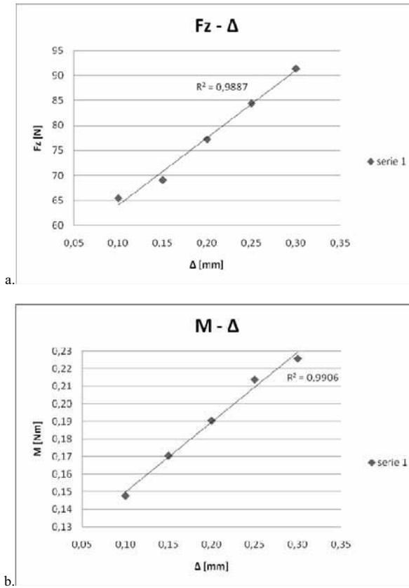
Fig. 3. (a) Influence of feed per revolution on feed force; (b) Influence of feed per revolution on cutting torque
