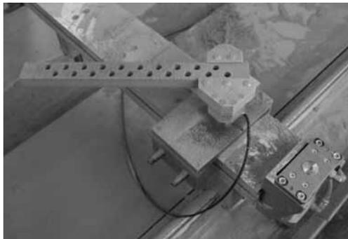
Fig. 2. Measuring platform with piezoelectric sensor and clamped sample
