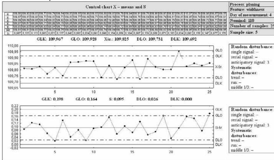
Fig. 5. Control chart for width dimension on day 4 of measurements
