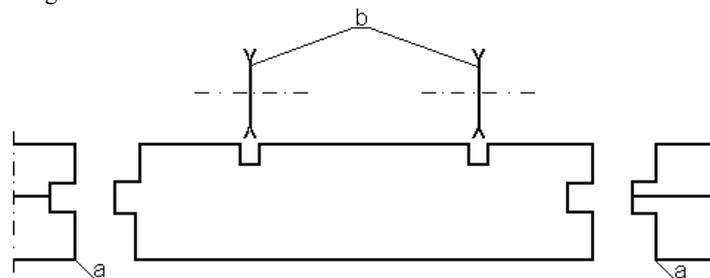
Fig. 2. Block diagram illustrating formation of sides and relief grooves of the floor board
