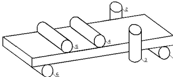
Fig. 1. Spindle arrangement of the applied type Unimat CLASSIC planing machine; 1, 6 – heads forming the top side of boards, 2, 3 – tongue and key profile milling cutters; 4 - disc cutter for relief grooves, 5 – head forming the bottom side
