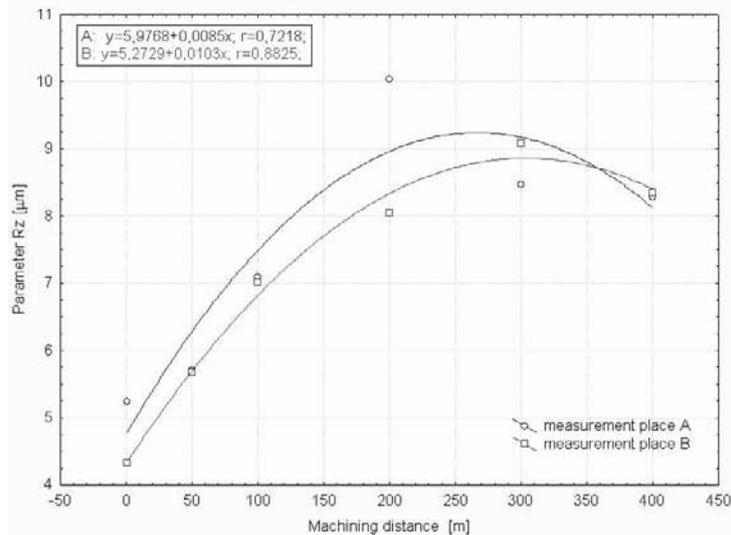
Fig. 4. Average peak to valley roughness Rz of the profile depending on the machining distance of the tool for the analysed measurement places.
