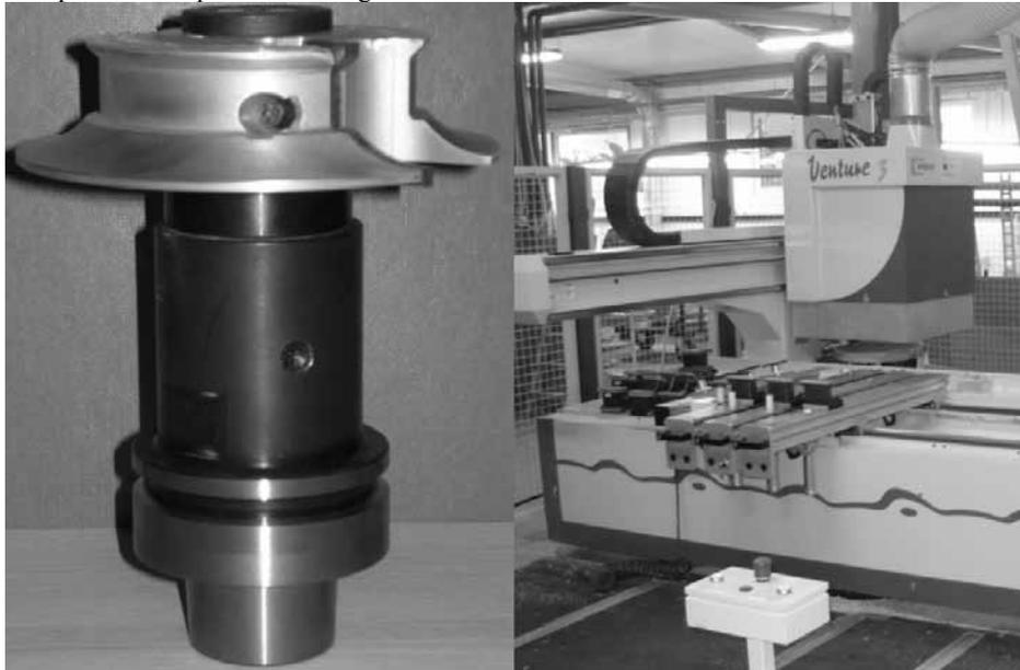
Fig. 1. Cutterhead and CNC woodworking machine employed in experiments
