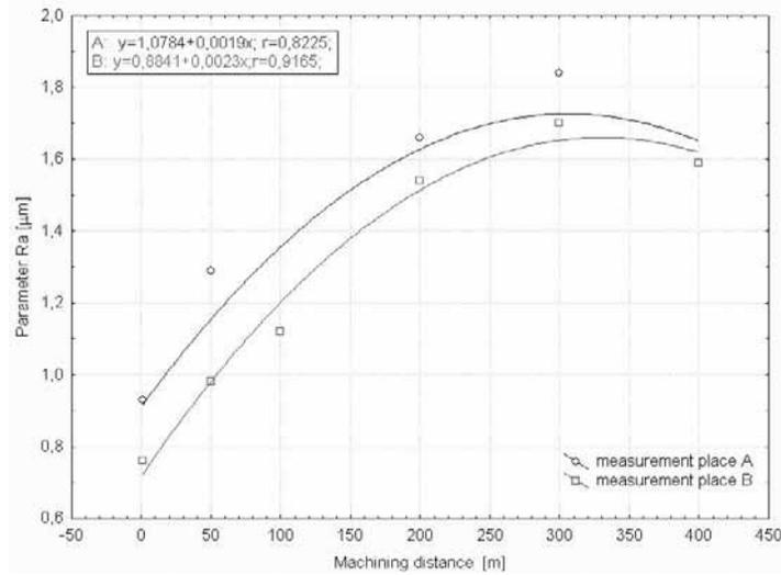
Fig. 3. Arithmetic average height Ra of the profile depending on the machining distance for the analyzed measurement places
