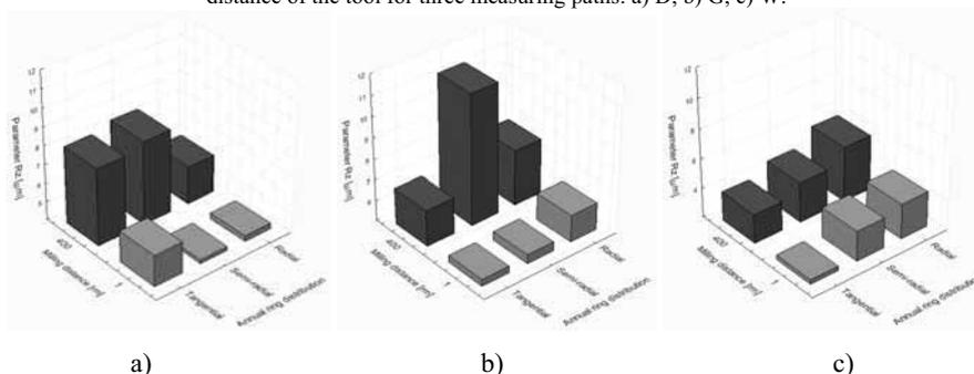
Fig. 5. Average peak to valley roughness Rz of the profile unevenness depending on the distribution of annual rings and the milling distance of the tool for three measuring paths: a) D, b) G, c) W.
