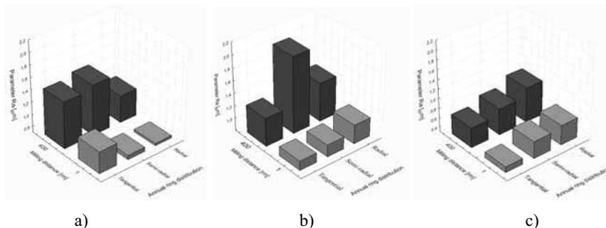
Fig. 4. Arithmetic average height Ra of the profile depending on the distribution of annual rings and the milling distance of the tool for three measuring paths: a) D, b) G, c) W.
