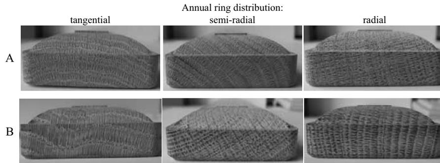
Fig. 2. Samples prepared for experiments: A – samples after processing with a sharp blade; B - samples after processing with a worn blade.
