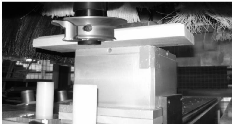
Fig. 1. Cutterhead and sample during milling.
