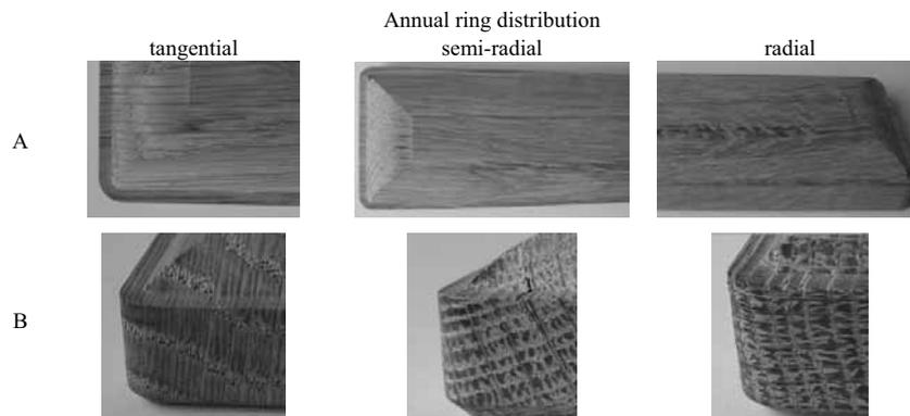
Fig. 6. Effects of burns of the examined samples: A – straight sections; B – corners
