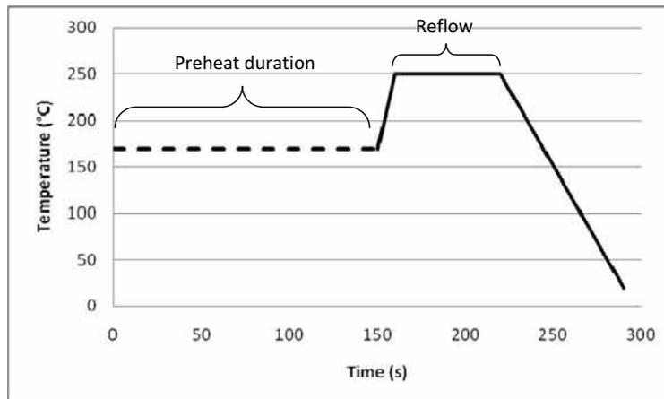
Fig. 2. Soldering profile with 150 s of preheating
