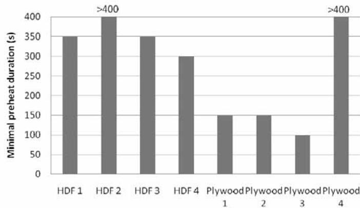
Fig. 4. Minimal preheat time at 170°C at the process causing solder to melt
