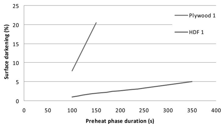
Fig. 5. Chosen WBPCB surface darkening after complete heating process with different phase duration
