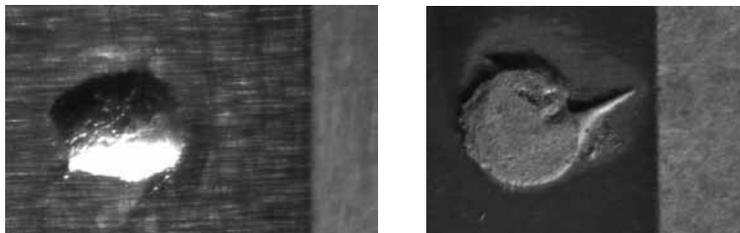
Fig. 3. Solder after WBPCB heating: a) well soldered joint, b) not fully melted solder
