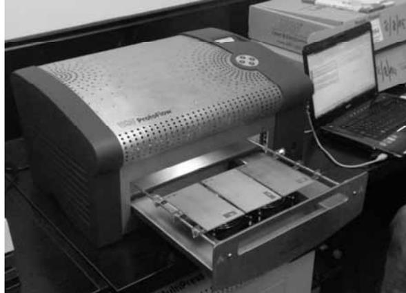
Fig. 1. Convection Lead-Free Reflow Oven used in experiments
