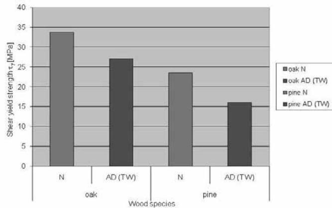
Fig. 2. Comparison of shear yield strength of pine and oak for both methods of drying: natural (N) and accelerated (AD) in the kiln
