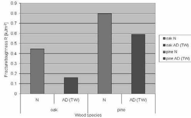
Fig. 1. Comparison of fracture toughness  $R$  of oak and pine, where: N – natural drying in air, AD – accelerated drying in the kiln
