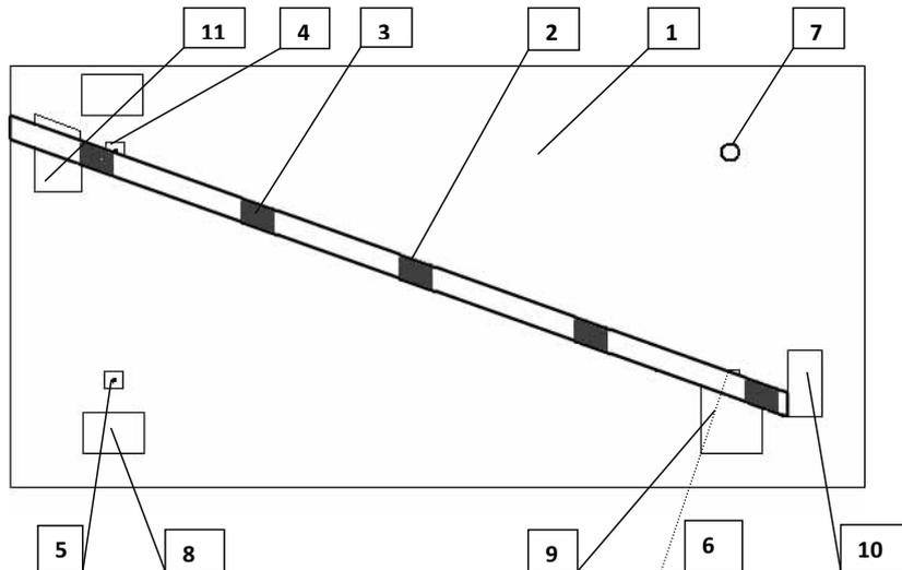
Fig. 1. The scheme of the measurement's station (1- reference plane, 2- measurement strip, 3- measurement area, 4- top constant peg, 5- left bottom peg, 6- right bottom peg, 7- top adjustable peg, 8- left block that hold sample during measurement, 9- left block that hold measurement strip and sample during measurement, 10- block, which the sample is levelled with, 11- top block that hold the measurement strip)
