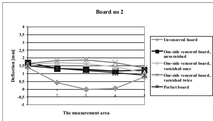
Fig. 4- The graph that shows deflection of the board that was asymmetrically veneered with using BISON TR550
