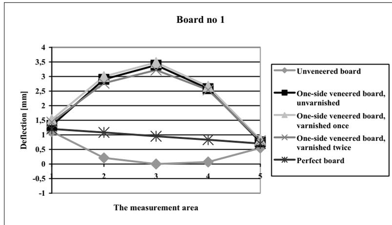
Fig. 3- The graph that shows deflection of the board that was asymmetrically veneered with using MULTIBOND2015
