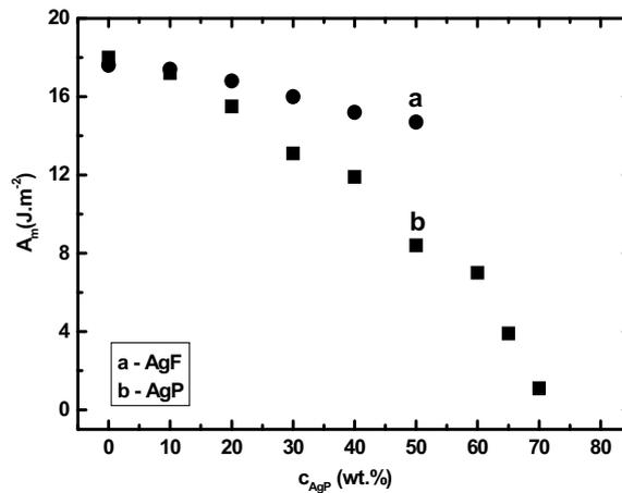
Fig. 2 Strength of adhesive joint of PSA composite to aluminium vs. content of the silver-coated filler: a – silver-coated wollastonite fibres, b – silver-coated basalt particles
