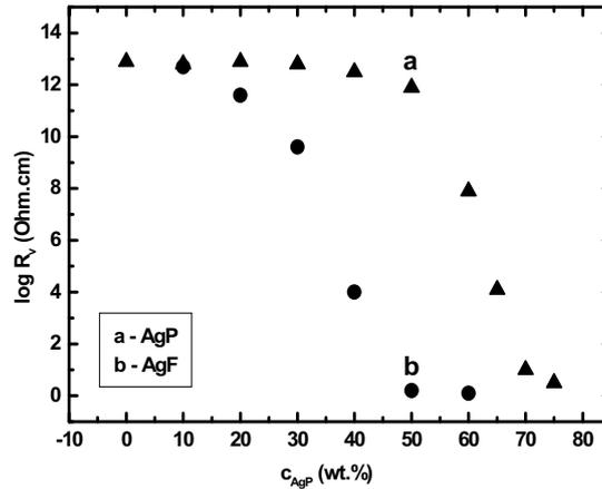
Fig. 1 Volume electrical resistivity of PSA composite vs. content of plated filler: a – silver-coated basalt particles, b – silver-coated wollastonite fibres
