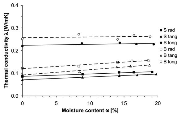
**Figure 2** Thermal conductivity ( $\lambda$ ) of Norway spruce (S) and European beech (B) in the radial (rad), tangential (tang) and longitudinal (long) directions depending on moisture content ( $\omega$ ). Linear regressions of Norway spruce (solid) and of European beech (dashed).
