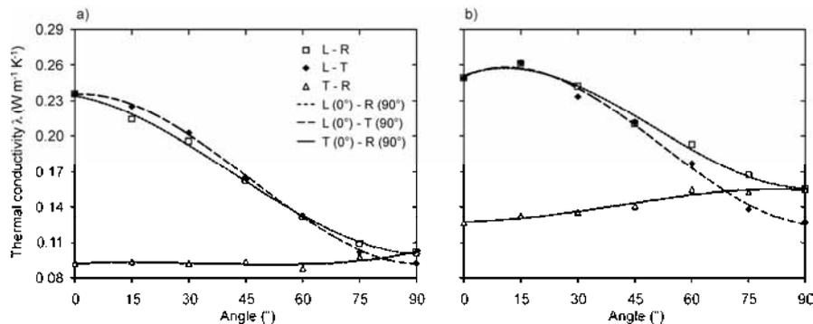
**Figure 3** Thermal conductivity ( $\lambda$ ) at 10°C in and between the principal anatomical directions of Norway spruce (a) and European beech (b) previously conditioned at 20°C and 65% RH. R = radial, T = tangential, L = longitudinal, points = measured data, lines = calculated values.
