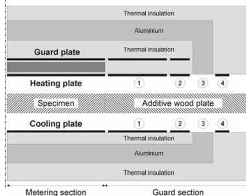
**Figure 1** Simplified half-diagram of the single-specimen guarded hot plate apparatus. 1, 2, 4 are the inner, middle and external heating guard rings and 3 the cooling ring (or tempering ring) to protect the test specimen from environmental influences.
