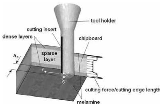
Fig. 1. Characteristic chipboard structure and cutting force distribution on the cutting edge in
