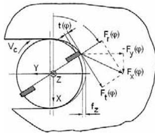
Fig. 2. Cutting forces in milling
