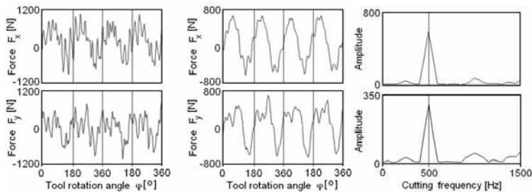
Fig. 3. Cutting forces signal in X-, Y directions before and after filtering
