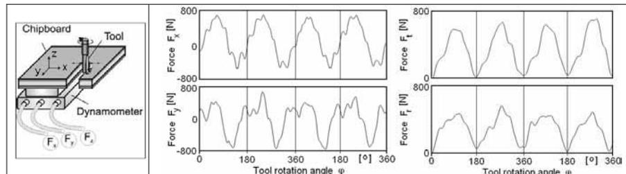
Fig. 4. Characteristic cutting force distribution on the cutting edge in chipboard milling
