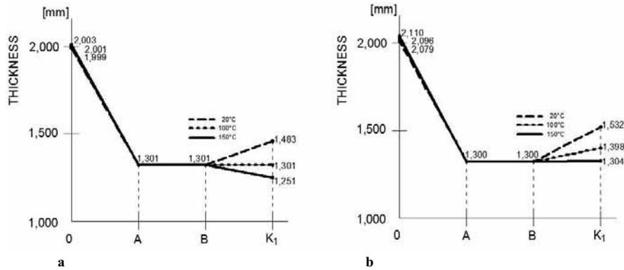
Fig. 3 The change of veneer thickness during pressing by 35% degree of pressing
