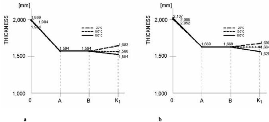
Fig. 2 The change of veneer thickness during pressing by 20% pressing degree
