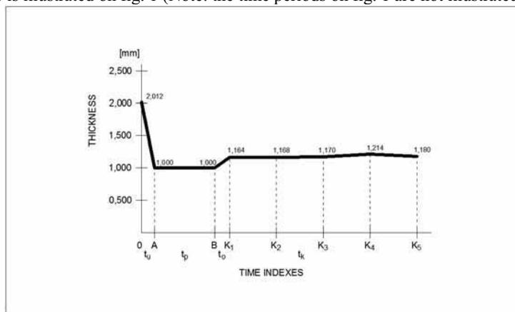
Fig.1 The change of veneer thickness during pressing and climatization by parameters mentioned in text
