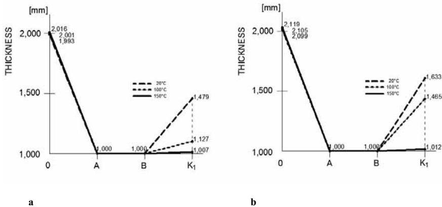
Fig. 4 The change of veneer thickness during pressing by 50% degree of pressing
