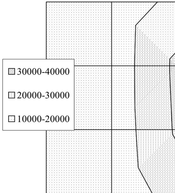
Fig. 1b Chromium concentration gradient in the pine wood sample for the assumed retention of  $1 \text{ kg/m}^3$  3 mm from the right sample front
