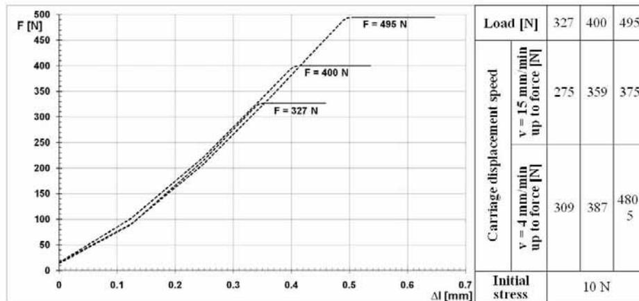
Fig. 2. The characteristics and parameters of creep tests
