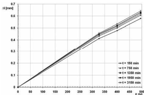
Fig 5. Isochronous creep curves obtained during tests of furniture joints elements
