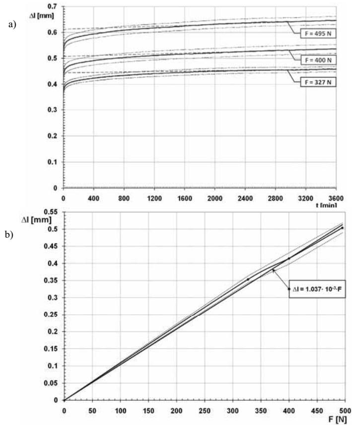
Fig 3. (a) the obtained creep curves; (b) the dependence of immediate displacement on load
