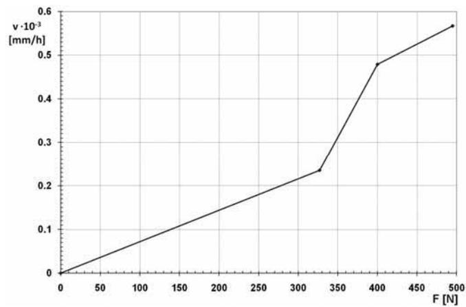
Fig 4. Dependence of average creep speed (between 54 and 60 tests hours) from load
