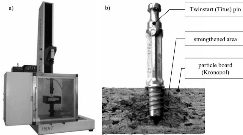
Fig. 1. (a) Tinus Olsen H5K-T universal testing machine with equipment; (b) tested specimen (dimensions 100x90x18).
