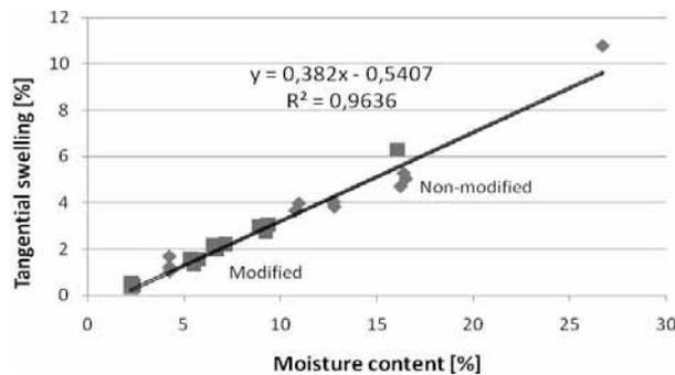
Fig. 3. The degree of wood swelling in the conditions of air humid versus its equilibrium moisture content
