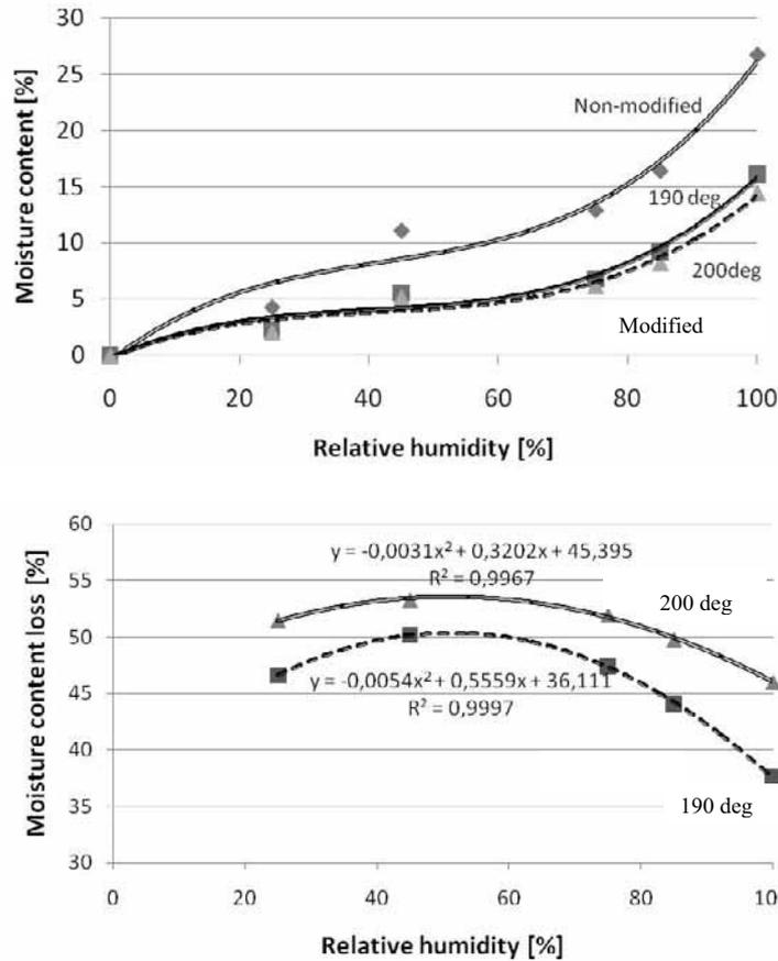
Fig. 1. The effect of thermal treatment of American ash wood on its equilibrium moisture content at different relative air humidity values
