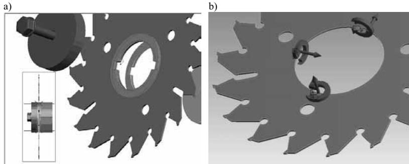
Fig. 1. Attachment of the saw blade: a) with collars, b) with take of the six degrees of freedom on the outside diameter of collars
