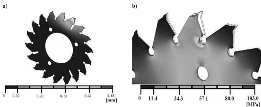
Fig. 3. Results of the calculations in the form of visualization: a) displacement, b) stress
