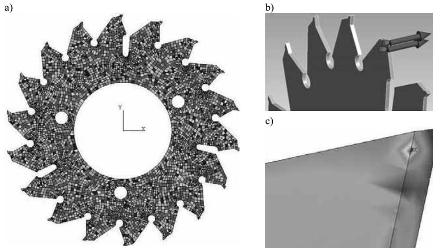
Fig. 2. Modeling of saw blade: a) divide of finite elements, b) loading the blade, c) effect of stress calculation, in the case concentrated force loading
