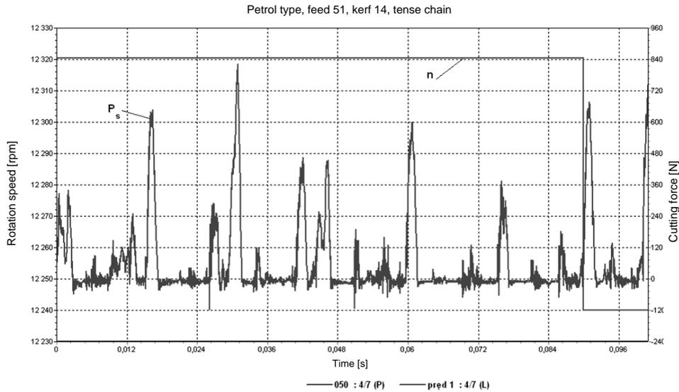
FIGURE 4. Variability of the cutting force at the feeding force of 51 N
