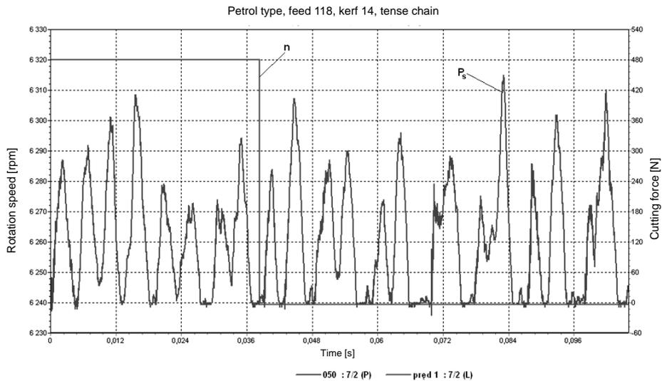
FIGURE 7. Variability of the cutting force at the feeding force of 118 N
