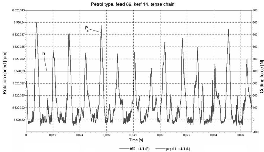
FIGURE 6. Variability of the cutting force at the feeding force of 89 N
