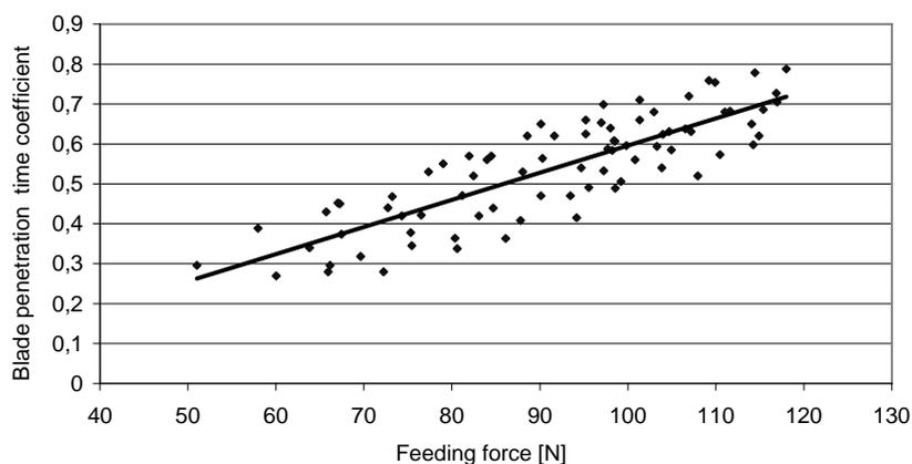
FIGURE 8. Influence of the feeding force on the blade immersion time coefficient
