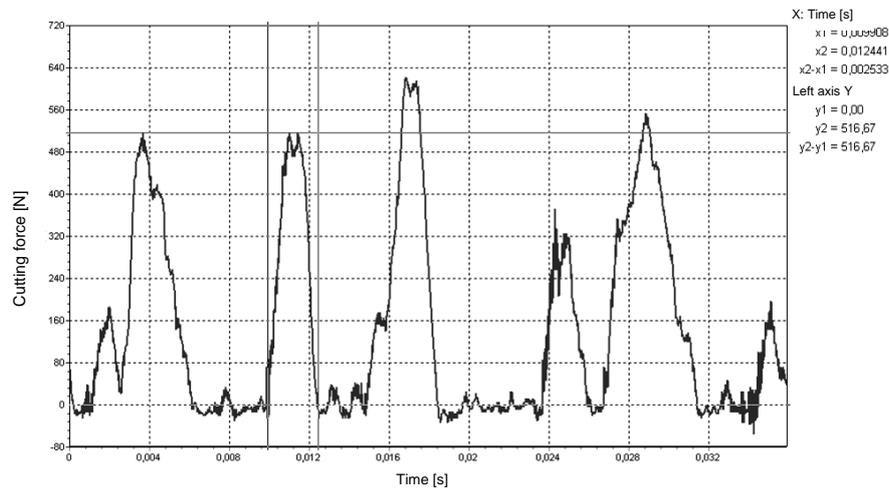
FIGURE 2. A fragment of the cutting force record of time length of 0.036 s:  $t_i$  – duration of the single immersion of saw chain cutters into the wood
