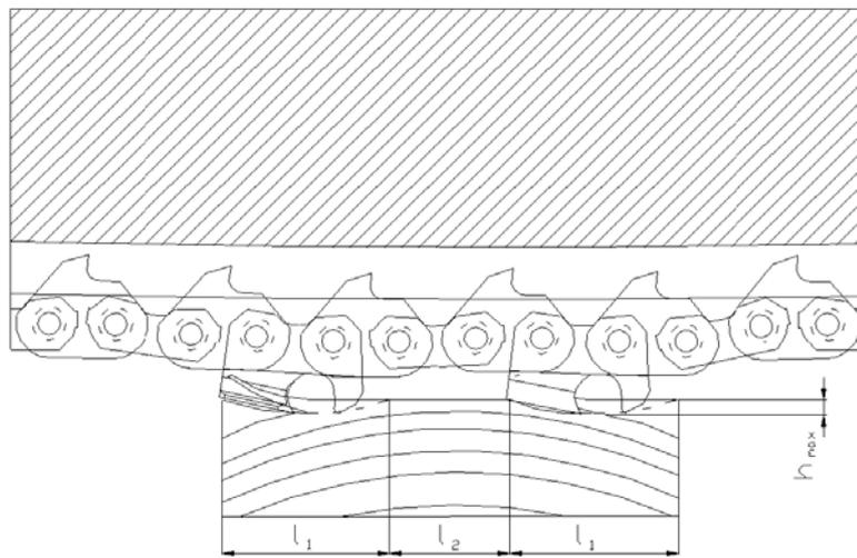
FIGURE 3. The course of the process of wood cutting with a saw chain:  $h_{max}$  – maximum chip thickness,  $l_1$  – distance covered by cutter inside the wood,  $l_2$  – distance covered by cutter outside the wood
