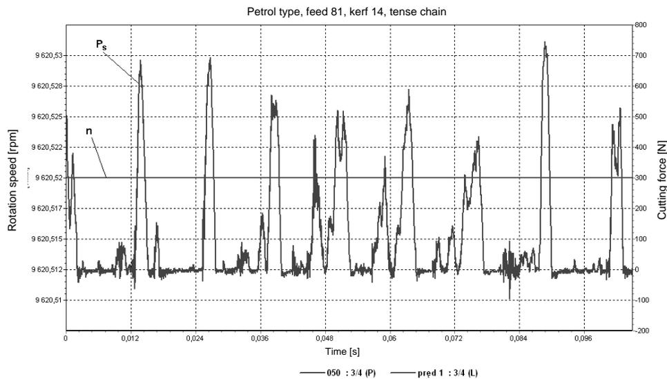
FIGURE 5. Variability of the cutting force at the feeding force of 81 N
