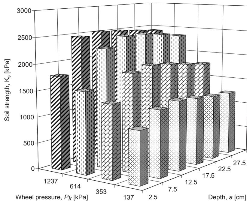
FIGURE 3. Soil strength changes resulted from compacting by wheel pressures
