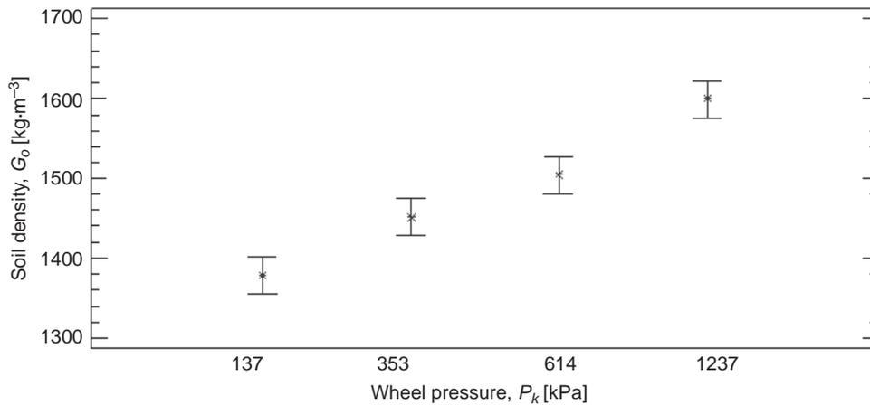
FIGURE 2. Average soil density values in the profile under track in particular measuring variants with confidence interval according to 95% HSD Tukey method
