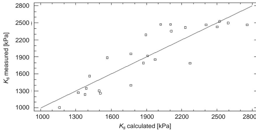
FIGURE 5. Comparison between values of strength ( $K_s$ ) calculated with equation and measurement values
