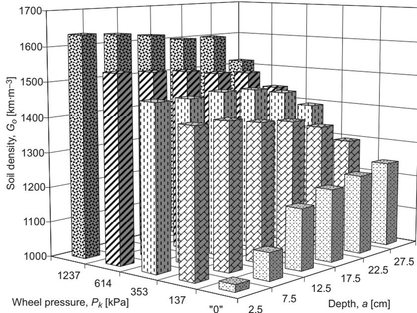
FIGURE 1. Soil density in the track for particular wheel pressure values
