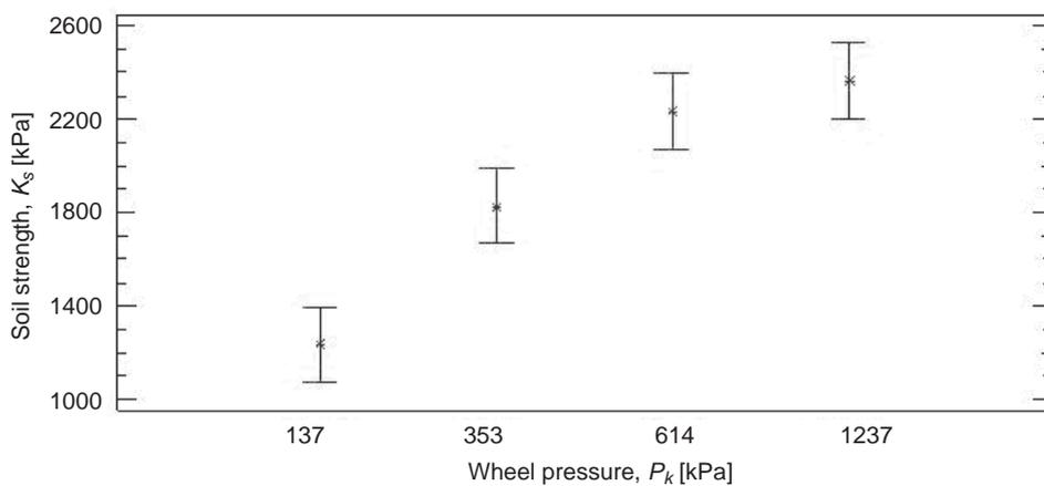
FIGURE 4. Changes in average soil strength in investigated profile as influenced by specific pressures
