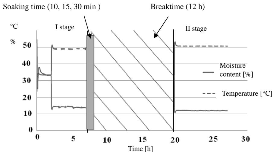
FIGURE 1. Changes in dry thermometer temperature and moisture content inside drying chamber, with marked soaking time and break for cones of II group
