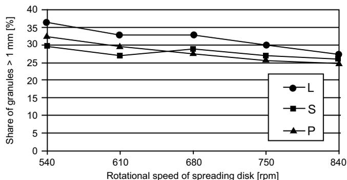
FIGURE 1. Effect of rotational speed and setting angle of vanes on the share of granules above 1 mm
