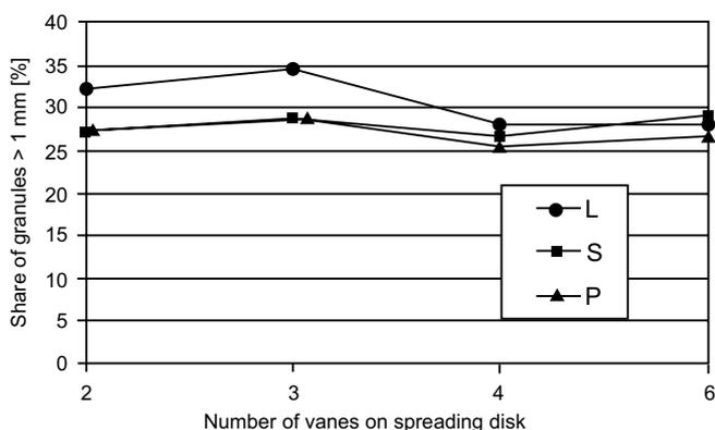
FIGURE 2. Effect of number of vanes and their setting angle on the share of granules above 1 mm
