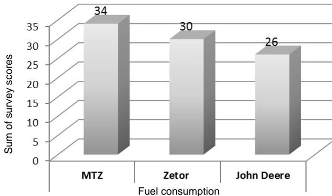
FIGURE 2. Results of investigations on fuel consumption of investigated tractors
