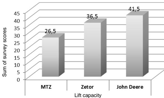
FIGURE 3. Results of investigations on lift capacity of investigated tractors
