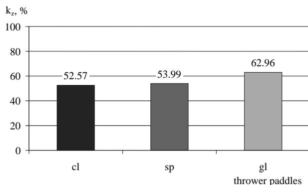
FIGURE 2. Average values of maize grain breaking-up index for various thrower paddles: cl – beater paddle with left hand bevel of notches, sp – beater paddle with right hand bevel of notches, gl – plain paddle
