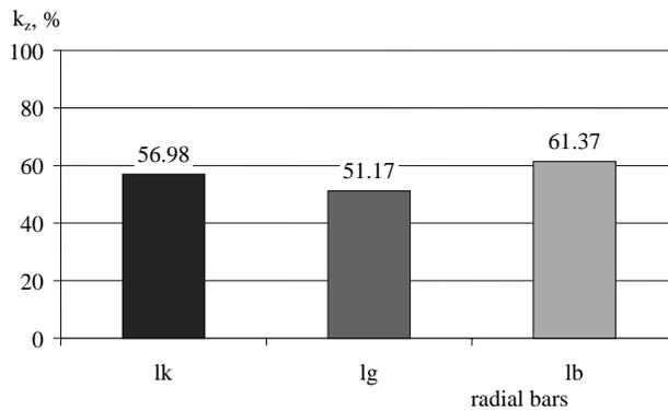
FIGURE 3. Average values of maize grain breaking-up index for various radial bars: lk – notched bar, lg – plain bar, lb – no bar
