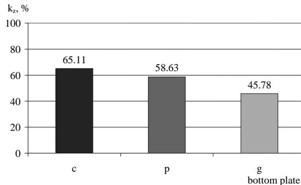
FIGURE 1. Average values of maize grain breaking-up index for various bottom plates: c – beater plate, p – rod plate, g – plain plate
