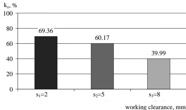
FIGURE 4. Average values of maize grain breaking-up index for various working clearance between bottom plate and thrower paddles
